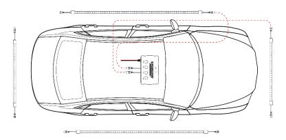
Note: There are two male plugs coming out of the control box. Ensure that you have one male plug from the control box plugged into the female end of the driver side tube and the other male plug from the control box plugged into the female end of the front tube. Each underbody tube daisy chains to the next with the included 6 feet of power wire and modular connectors.
