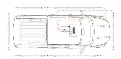
**Note:** There are two male plugs coming out of the control box. Ensure that you have one male plug from the control box plugged into the female end of the driver side strip and the other male plug from the control box plugged into the female end of the front strip. Each underbody strip daisy chains to the next with the included 6 feet of power wire and modular connectors.
