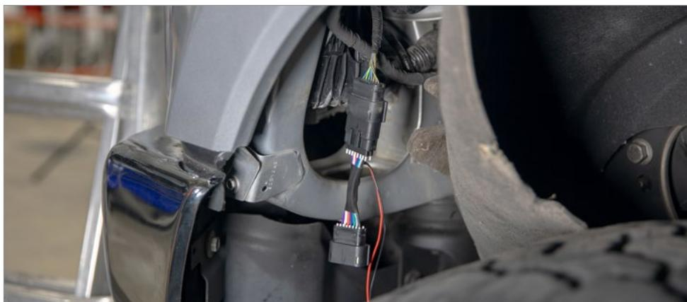
16. Route the wires from the pass-through harness behind the grille and plug in the grille light splitter harness.
