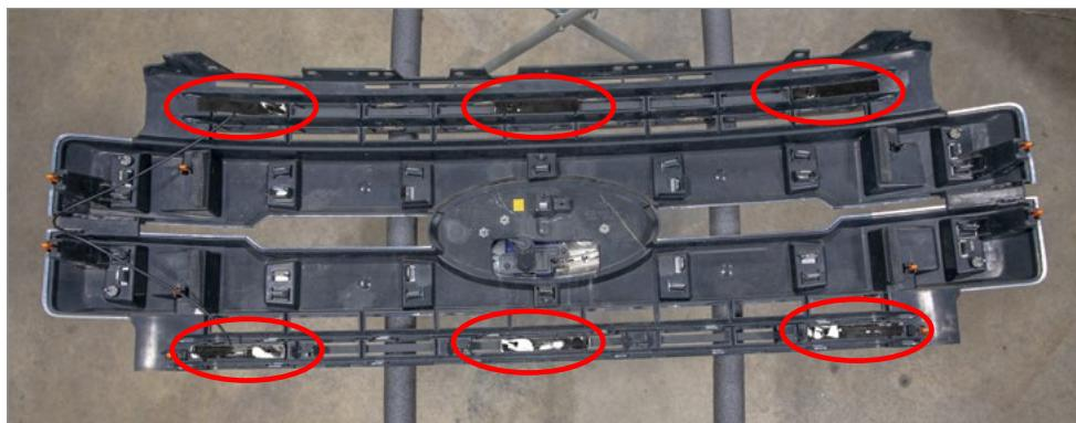
11. Tighten the nuts on the light bar using a 5.5mm socket.
