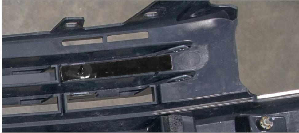
8. Tighten the nuts on the light bar using a 5.5mm socket.
