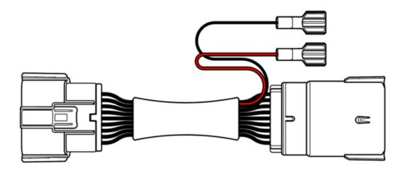
**Note:** This add-on harness is designed to easily integrate 12-volt accessories controlled by the vehicle's running lights. For a larger amp-draw accessory, a relay must be installed to supply adequate voltage to the accessory.
