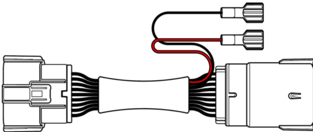
**Note:** This add-on harness is designed to easily integrate 12-volt accessories controlled by the vehicle's running lights equipped with factory LED headlamps. For a larger amp-draw accessory, a relay must be installed to supply adequate voltage to the accessory.
